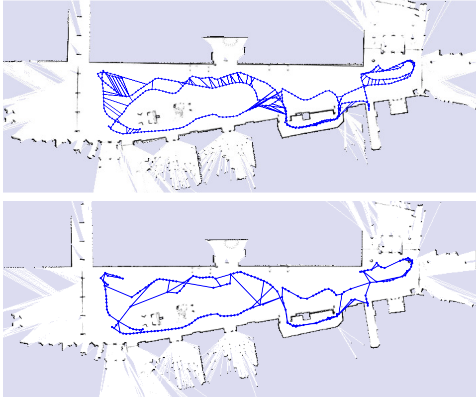
Figure 7: Map and pose graph obtained when mapping the FR101 dataset. Top: Standard approach, 408 nodes, 723 edges. Bottom: Our approach, 200 nodes, 246 edges. Since the robot does not frequently re-traverse previously visited terrain, few scans were discarded.
