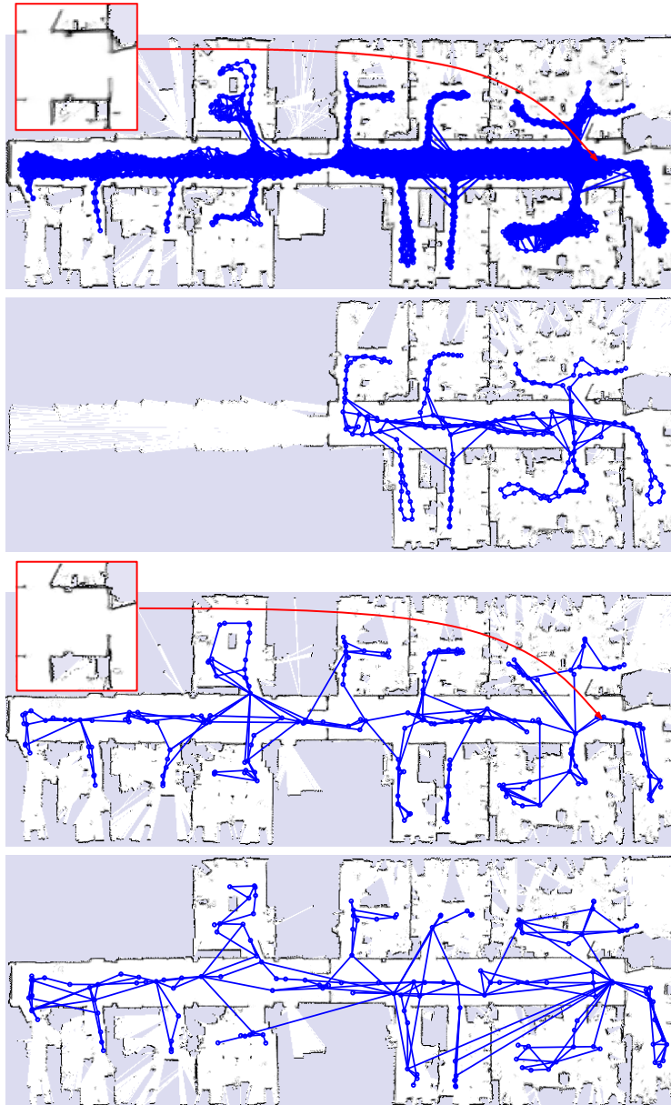
Figure 6: The robot moved around in an office environment for an extended period of time, visiting the rooms and the corridor many times. First: Standard approach, 2597 laser scans, 15695 edges. Second: Our approach at an intermediate time step, 200 laser scans, 264 edges. Third: Our approach, 200 laser scans, 315 edges. Fourth: Our approach when setting a threshold for the mutual information, 148 laser scans, 250 edges instead of a fixed value.
