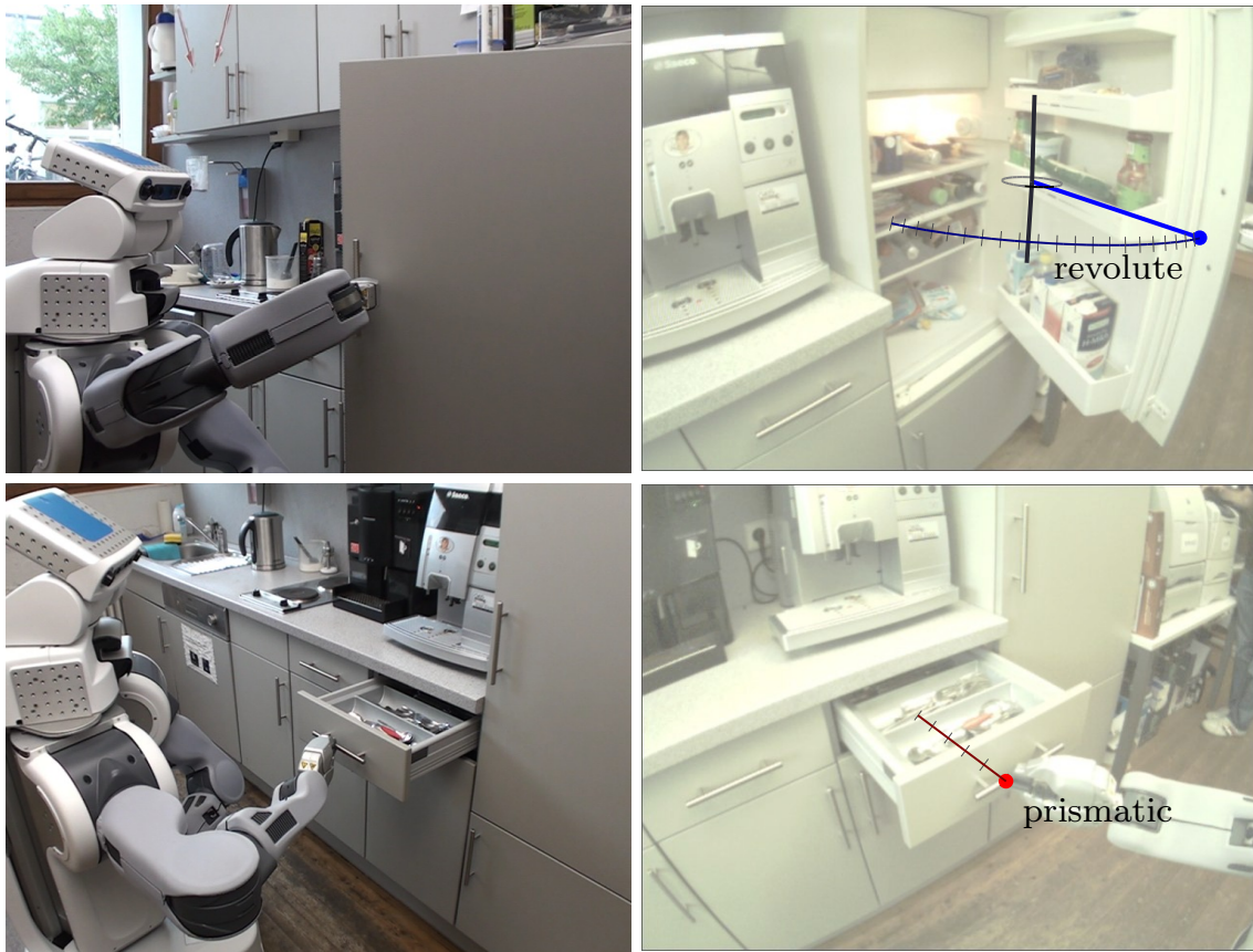
Figure 1: A service robot learns kinematic models of articulated objects in a kitchen environment.
