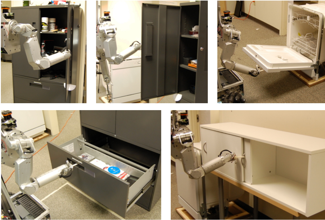
Figure 15: Images showing the robot Cody at Georgia Tech operating the five mechanisms using the approach described in Section 4.3. The objects are (from left to right): a cabinet door that opens to the right, a cabinet door that opens to the left, a dishwasher, a drawer, and a sliding cabinet door. Images courtesy of Jain and Kemp.
